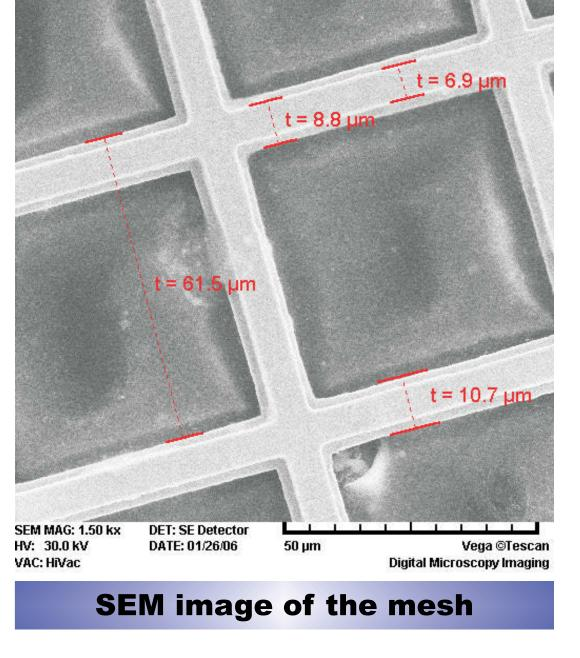
Azoom-in on a detail of the grid is shown in Fig 4. It shows that the resolution of the imaging system is in the order of micrometers.
